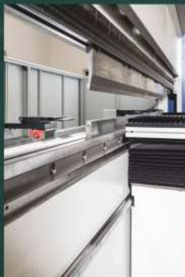
600 mm daylight (G-series). Wila tooling.
