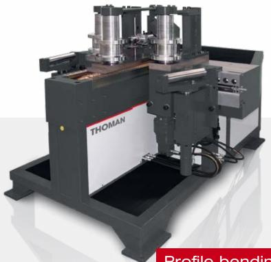
Profile bending machine RB4
