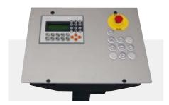
It doesn't always have to be CNC. As an alternative to CNC-S control, the type RB profile bending machines are also available as an NC controlled version with one or two controlled axes.
